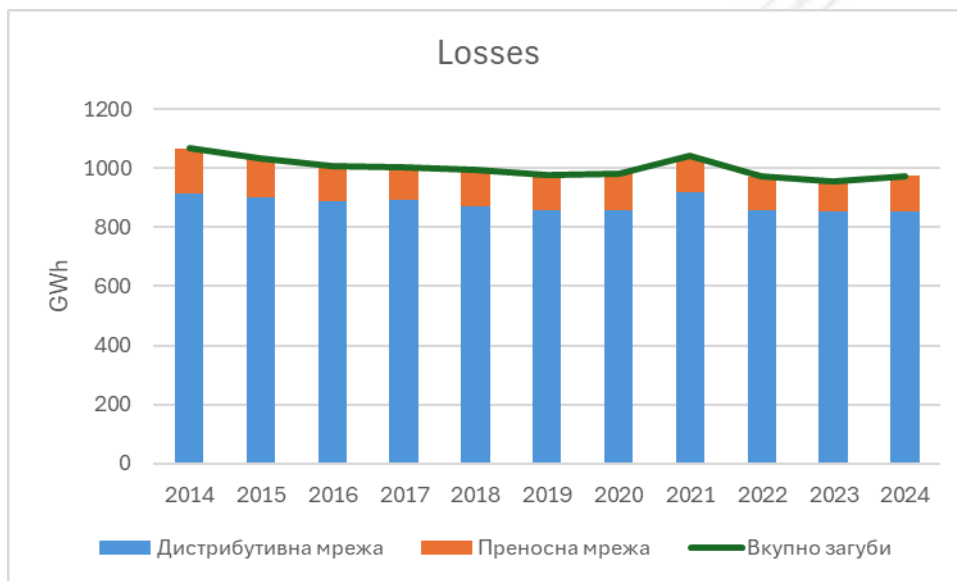
Figure 4. Losses on transmission and distribution network
